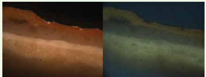
Fig. 3/4 – (Left) Cross-section scan of gold on the moldings. (Right) Ultraviolet scan. Copyright Helen Hughes: Historic Interiors Research & Conservation, London.
